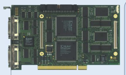
HORIZON LINK board is an i2S multi channel PCI board, designed to easily interface Camera Link™ Line scan cameras.
